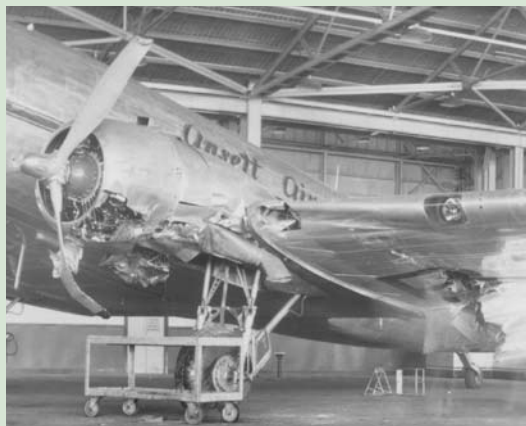
An Ansett DC3 after it had crashed into a goods train on the old strip at Mascot
