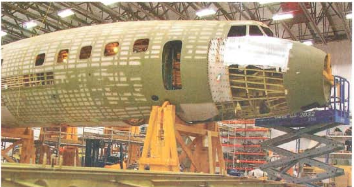
The fuselage of the Lockheed L1649A Starliner being restored in the USA for the Lufthansa Historic Flight. It is expected to return to flight status in 2012.
