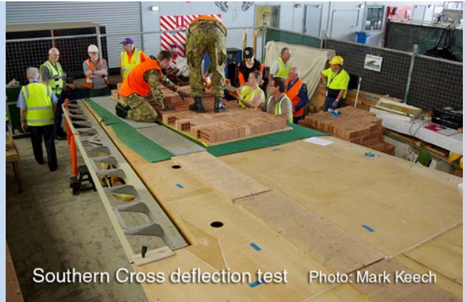
Southern Cross deflection test Photo: Mark Keech
